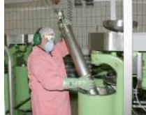
Fig 1: Pulling out the rotor with a ceiling mounted lifting tool.
